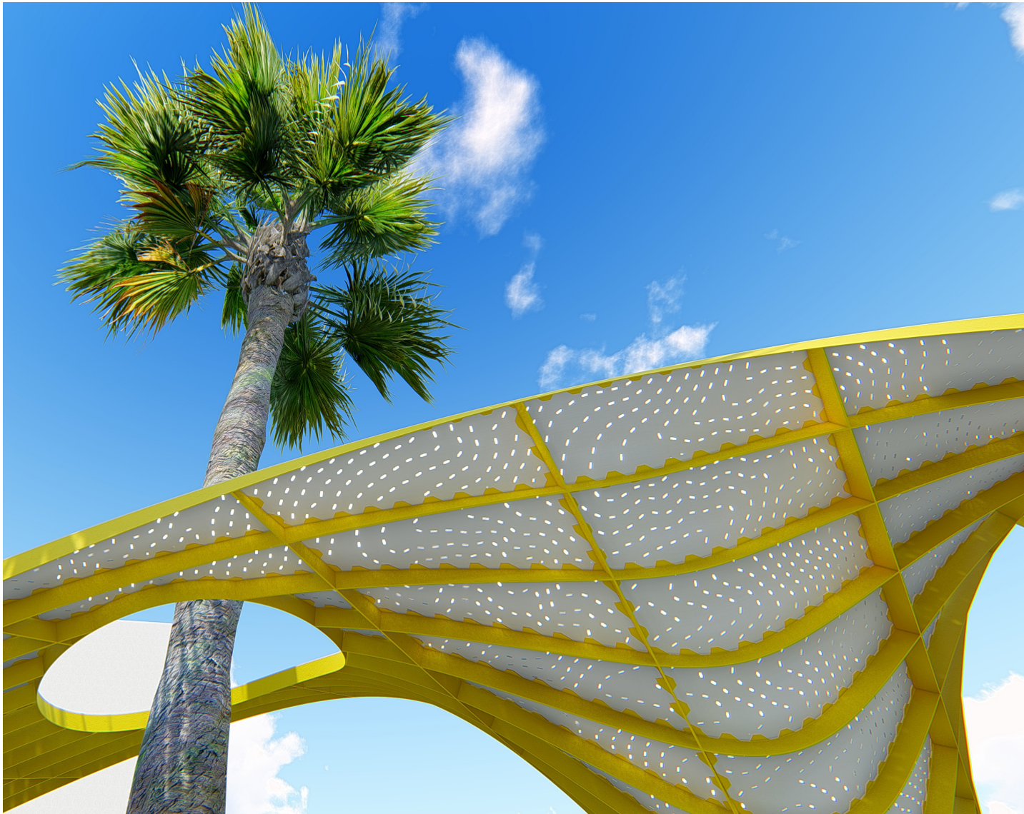
Panels are prefabricated and partially assembled at the foundry. Depending on further structural evaluation the panels would be made of stainless steel, powder coated aluminum or a combination of the two .
